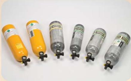
MSA offers a choice of three low-pressure (2216 psig) 30-minute-rated cylinders for use with this SCBA. Choose carbon-wrapped, fiberglass hoop-wound, or all-aluminum construction cylinders. High-pressure (4500 psig) carbon-wrapped cylinders are available in 30-, 45-, or 60-minute durations.
